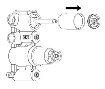
Using an adjustable spanner, unscrew the Flow Collar and remove the seal. There are flats on the back for the adjustable spanner to grip on to.
