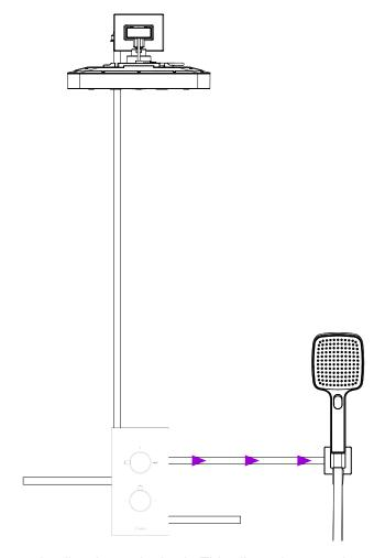
With the Flow Cartridge reversed, the water will flow out in the opposite direction to the knob. This allows the artwork to match the water outlet with the Hand Shower.
