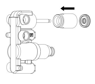
Remove the Flow Cartridge, turn it 180° and place it back inside the valve. Use the 2 locator pins on the back of the Flow Cartridge to make sure it is secured.
