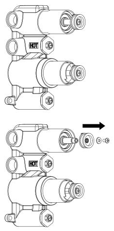
Unscrew the top screw and remove the washer and Flow Adaptor.
