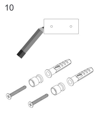
Use the cut out on page 28 to mark out and drill the holes for the Handset Holder. Then Place the Wall Plugs inside the holes and screw the Mounting Brackets onto the wall using the Wall Screws.
