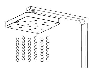
Run the showerhead with power to test the air and water supply. We recommend running this test at 38°C. Please note the bubbles do not form as consistently below 20°C. Once you are satisfied with the bubbles, remove the protective film from the faceplate and enjoy your BubbleSpa® shower.
