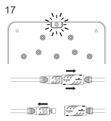
Once the power is turned on, the Button Light on the showerhead will light up. This is an indicator that power is being supplied to the showerhead. If you need to disconnect the power cable, first isolate the mains. Then pull back the outer layer of the larger connector then remove the small connector.
