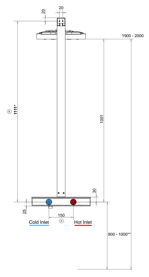
$<sup>^{*}</sup>$ This is a critical dimension. The holes at the top are slots allowing for variance of +/- 5mm.
