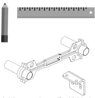
Refer to the measurements on page 10 and mark out the holes for the outlet pipes [A] and the Wall Bracket [B]. Use the Alignment Tool to assist with marking the holes for the Fixing Brackets. Referring to the measurements on page 10, mark the holes where the Wall Bracket [B] will be. Use the Alignment Tool to help mark out the holes for the Fixing Bracket.
