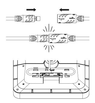
Switch off the water then attach the Power Cable by aligning the 2 arrows on the connectors and then pushing the connectors together until a click is heard. Then place the cables into the clips on the Overhead Shower. Connect the other end of the power cable to the Transformer. Then turn on the power supply to the Overhead Shower from the mains.
