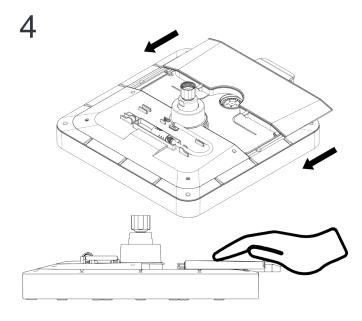
Slide the Dust Cap onto the Overhead Shower. Make sure the Dust Cap is secured tightly and then mount the Overhead Shower onto the arm using a spanner. Reconnect the power cable then switch on the power and water supply.
