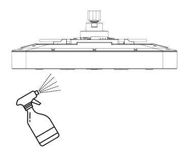
Spray cleaning solution onto the faceplate.
