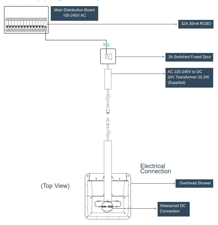
The BubbleSpa® Overhead Shower does not require its own [electrical port] on the RCB. Since the BubbleSpa® can be run from a port being used eg. a kitchen port or lighting. See next page for full details.
