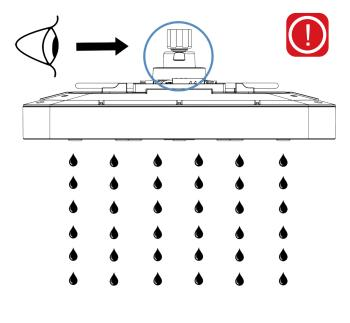
Run the Overhead Shower without power to test the water supply. Whilst the shower is running, check the entire installation for any leaks, especially the Ball Joint and Ball Joint Clamp (circled) of the Overhead Shower. It is important that there is no water leaking as this can damage the fan and PCB. Make sure to also check the mixer operation, the temperature and the flow rate.
