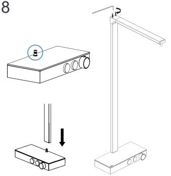
Feed the power cable of the Exposed Arm Assembly into the wall and route/fish the power cable through the wall towards the Transformer. Then apply plumber's silicone grease to the O-rings on the Shelf Mixer (circled) and place the Exposed Arm Assembly down onto the Shelf Mixer and on the Wall Bracket. Secure the Exposed Arm Assembly onto the Wall Bracket with the Retaining Screws.
