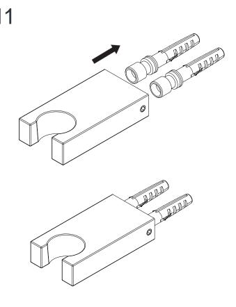
Place the Handset Holder onto the Mounting Brackets and secure it using the Mounting Grub Screw.
