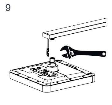
Screw the BubbleSpa® Overhead Shower onto the Exposed Arm Assembly. Use a 23mm spanner on the Ball Joint and a 28mm spanner on the Ball Joint Clamp.
