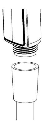
Screw the Hose onto the outlet on the underside of the Shelf Mixer. Make sure that there is a washer inside of the hose before fitting.
