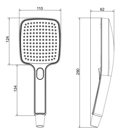
Tilting of the BubbleSpa® Overhead Shower can be in any direction. All dimensions are in mm unless otherwise stated.
