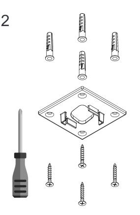
Insert the Wall Plugs provided into the ceiling and screw the Ceiling Arm Assembly using the screws provided.
