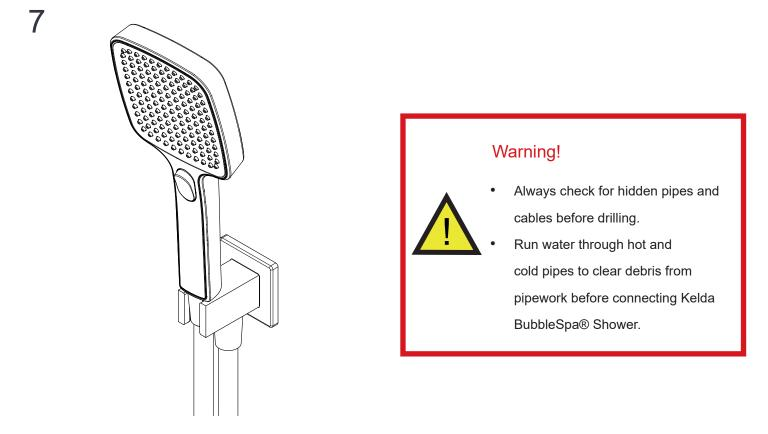
The installation of the Hand Shower is complete. Place the Hand Shower onto the mount.
