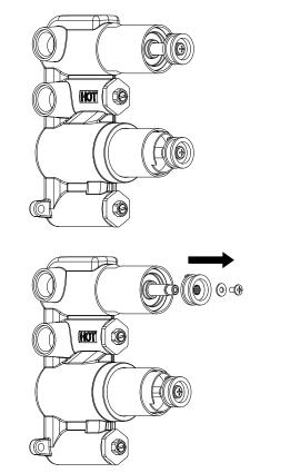
Unscrew the top screw and remove the washer and Flow Adaptor.
