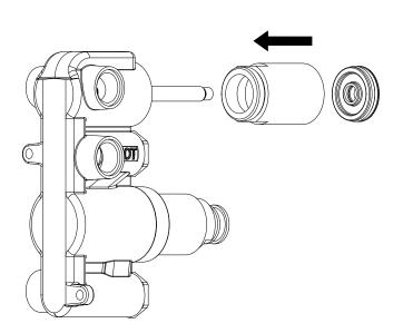
Screw the Flow Collar with the seal back into the valve using an adjustable spanner. Ensure the seal is pushed down the Flow Collar as far as it can go.
