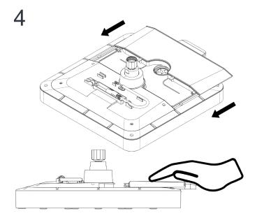
Dry the Dust Filters and place them back into the Dust Cap. Make sure the Dust Filters are secured tightly in the Dust Cap. Slide the Dust Cap onto the Overhead Shower. Make sure the Dust Cap is secured tightly and then mount the Overhead Shower onto the arm using a spanner. Reconnect the power cable then switch on the power and water supply.
