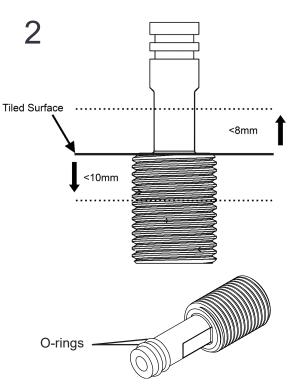
Screw the Water Path Connecter to the outlet pipe. Ensure that the Water Path Connector is no more than 10mm proud of the wall tiles and is no more than 8mm inside the wall. Apply plumber's silicone grease onto the O-rings on the Water Path Connector.
