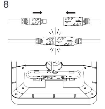
Switch off the water then attach the Power Cable by aligning the 2 arrows on the connectors and then pushing the connectors together until a click is heard. Then place the cables into the clips on the Overhead Shower. Connect the other end of the power cable to the Transformer. Then turn on the power supply to the Overhead Shower from the mains.
