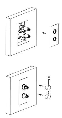
Re-fit the Knob Adapter, screw and washer by reversing step 2. Make sure the protrusion [circled above] points to the 12 o'clock position.
