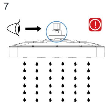
Run the Overhead Shower without power to test the water supply. Whilst the shower is running, check the entire installation for any leaks, especially the Ball Joint and Ball Joint Clamp (circled) of the Overhead Shower. It is important that there is no water leaking as this can damage the fan and PCB. Make sure to also check the mixer operation, the temperature and the flow rate.
