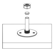
In the ceiling void, place the Mounting Plate over the inner tube. Attach the Mounting Plate to the plywood with Wall Plugs and Wall Screws provided. Then place the Olive and Compression Nut over the inner tube and tighten the nut.
