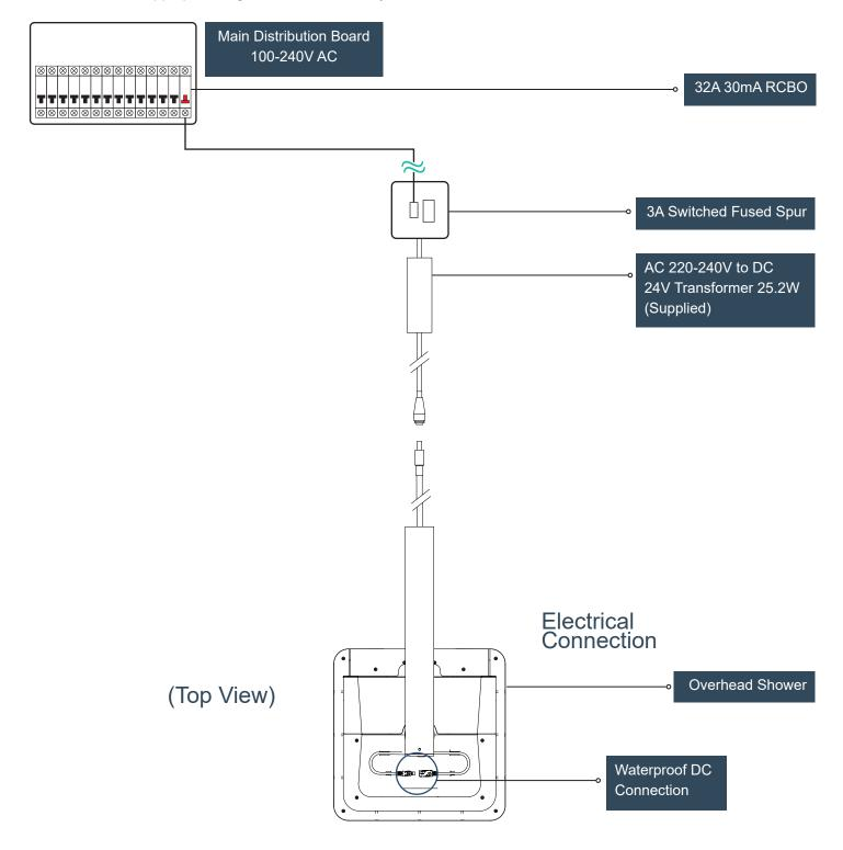
The BubbleSpa® Overhead Shower does not require its own [electrical port] on the RCB. Since the BubbleSpa® can be run from a port being used eg. a kitchen port or lighting. See next page for full details.
