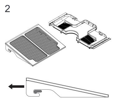
Remove the Dust Filters from the Dust Cap as shown and clean the Dust Filters. Wipe down the underside of the Dust Cap and the surface of the Overhead Shower with a damp cloth. Take care not to get any moisture on to the fan.
