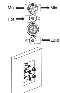
Determine the position of the valve and hold the valve inside the wall cavity. Mark out the fixing points for the screws. Remove the valve and drill in holes for the Wall Plugs. Secure the valve within the wall cavity using the Wall Plugs and Wall Screws.
