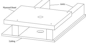
It is recommended to use a sheet of plywood supported by joists (as shown above) to fix the pipe mount permanently. Before installing, make sure the inner pipe of the Ceiling Arm Assembly is long enough to reach above the plywood sheet –cut the inner pipe if it is too long. Once the position of the shower has been determined, drill a hole that is bigger than 17mm but no larger than 60mm diameter in the ceiling.
