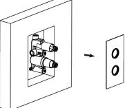
Unscrew the Knob Levers from the Grub Screws then unscrew the Grub Screws from the Control Knobs using the Hex Key. Remove the Control Knobs and remove the Kelda Faceplate.
