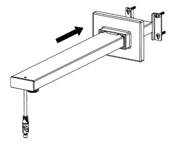
Feed the power cable of the Wall Arm Assembly into the wall and route/fish the power cable through the wall towards the power supply. Then screw the Wall Arm Assembly to the wall using the Wall Screws and Wall Plugs provided. Ensure that the O-rings on the Water Path Connector are not displaced.
