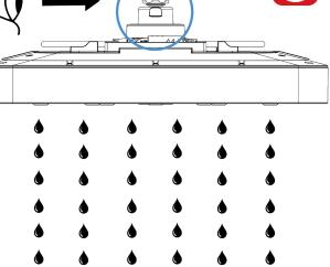
Screw the BubbleSpa® Overhead Shower onto the Ceiling Arm Assembly. Use a 23mm spanner on the Ball Joint and a 28mm spanner on the Ball Joint Clamp.
