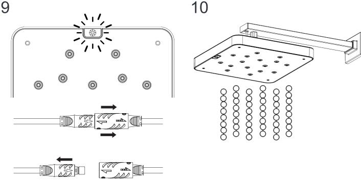
Once the power is turned on, the Button Light on the Overhead Shower will light up. This is an indicator that power is being supplied to the Overhead Shower. If you need to disconnect the power cable, first isolate the mains. Then, pull back the outer layer of the larger connector, then remove the small connector.
