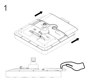
Switch off the water and power and disconnect the power cable on the Overhead Shower. Then dismount the Overhead Shower using a spanner and place the Overhead Shower onto a soft cloth. Be careful not to get any water onto the fan. Then slide the Dust Cap off the Overhead Shower as shown with both hands.
