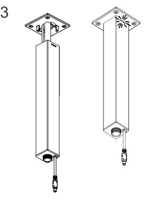
Feed the power cable of the Ceiling Arm Assembly into the void. Attach the Ceiling Arm Assembly to the Ceiling Arm Bracket. The Ceiling Arm Assembly will snap onto the bracket. The inner tube will go through the hole with sufficient length to attach the water supply. The inner tube may be cut to length if it is too long.
