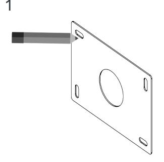
Using the guide provided on page 40, mark out and drill the holes for the Wall Arm Assembly around the pipe outlet. Ensure that the hole for the cable and outlet pipe is no bigger than 60mm diameter.
