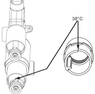
Re-fit the Temperature Control Ring with the [arrow] protrusion pointing to the 12 o'clock position.
