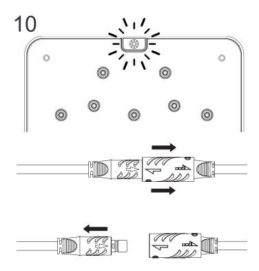
Once the power is turned on, the Button Light on the Overhead Shower will light up. This is an indicator that power is being supplied to the Overhead Shower. If you need to disconnect the power cable, first isolate the mains. Then pull back the outer layer of the larger connector then remove the small connector.
