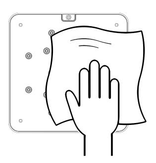
Wipe the faceplate using a damp cloth to remove the loosened debris.
