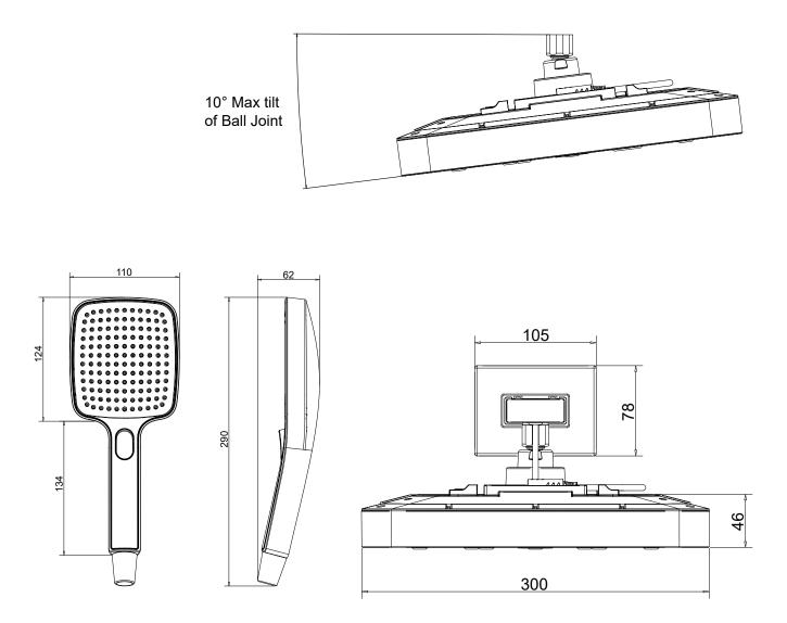
Tilting of the BubbleSpa® Overhead Shower can be in any direction. All dimensions are in mm unless otherwise stated.
