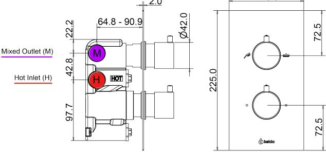
Inlets and outlets are all  $\frac{1}{2}$ " female threads. Minimum wall cavity depth: 83mm.
