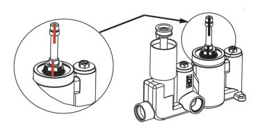
Keep the two marked lines in line whilst turning the spindle. Turn the spindle anti-clockwise to reduce the water temperature (or turn the spindle clockwise to increase the temperature). Measure the temperature of the water and adjust as required. Be careful not to get any water into the wall cavitiy.
