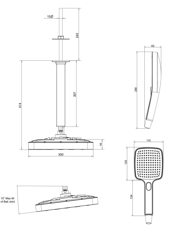
\*Drawing shows the lengths of the parts as supplied. The Inner Pipe can be cut down to an appropriate length if necessary. The tilting of the BubbleSpa® Overhead Shower can be in any direction. All dimensions are in mm unless otherwise stated.
