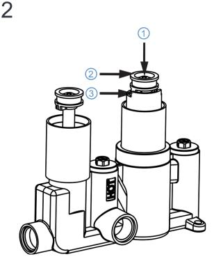
Remove the screw & washer [1], the Knob Adapter [2] and Temperature Control Ring [3] from Thermostatic Cartridge.
